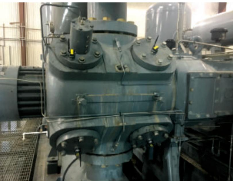
■ Vibration sensors with wireless transmitters are attached to the suction and discharge valve caps.
