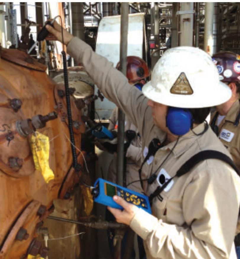
■ A technician uses an ultrasound needle sensor to test for problems.
